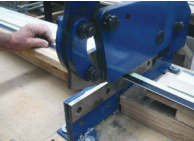
Using guillotine (hand shears) to cut strip
